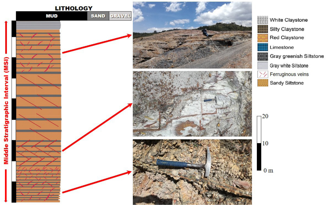
FIG. 6. Stratigraphic column of the MSI. In the middle picture, the iron oxide veins have two preferred orientations. The fossil content is typically poor. See figure 2 for column location.
