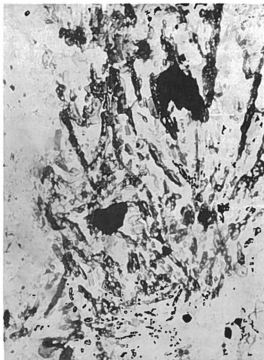
FIG. 9C Microphotograph (x 100) of a replacement clot, in the halo of a Type 4 vein. Andalusite, corundum and feldspar are present along with lesser amounts of brown micas.
