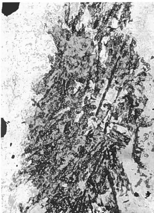
FIG. 9A Microphotograph (x 100) of a replacement clot, in the halo of a Type 4 vein, formed mainly by a fine-grained intergrowth of mostly brown biotite (low relief mineral), and andalusite (high relief mineral).
