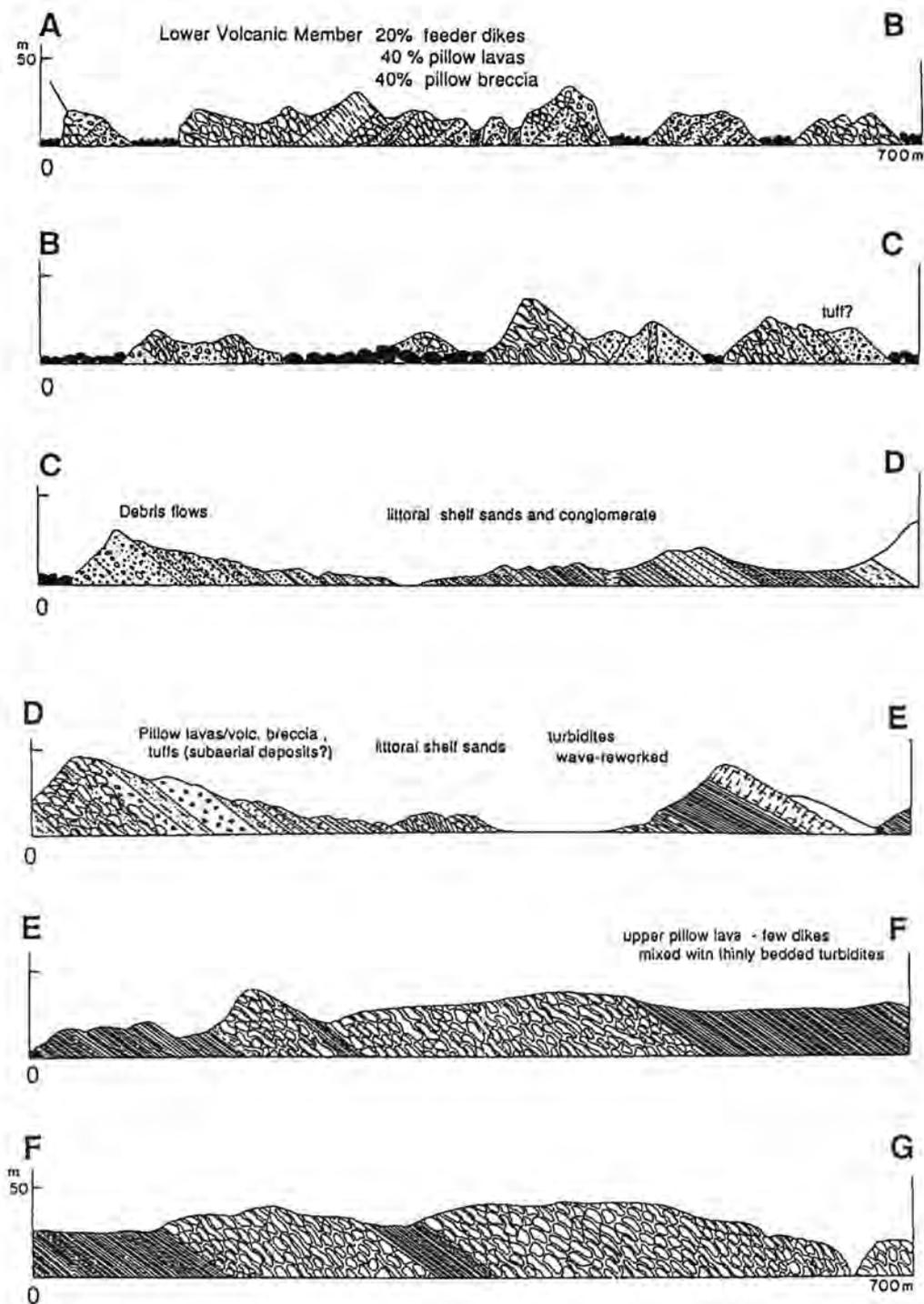
Text-FIG. 4. Geologic profiles constructed by zodiac reconnaissance from point A-G shown in text-figure 3. Topography of the coast is diagrammatic. Black areas indicate talus cover, cross-hatched areas indicate sea caves.
