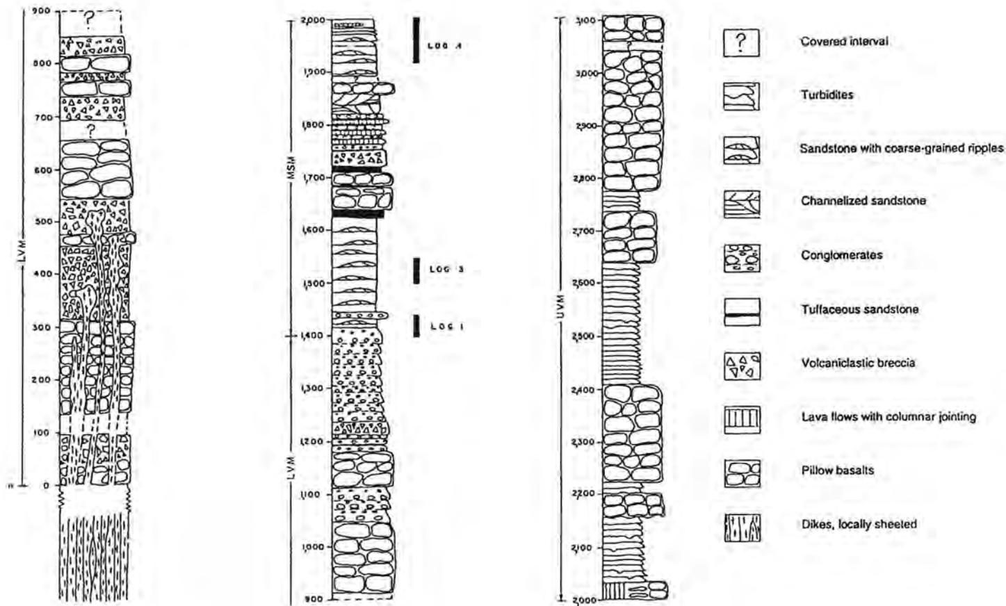
Text-FIG. 5. Generalized stratigraphic section of the Bahía San Andrés Formation divided into the three members: LVM= lower volcanic member; MSM= middle sedimentary member; UVM= upper volcanic and sedimentary member. The section was constructed using the profiles of text-figure 4. The positions of logs 1, 3, and 4 are indicated. Note: thicknesses are approximate and may be up to 15% too thick.
