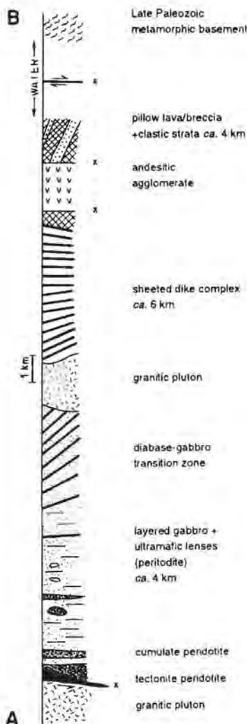
Text-FIG. 8. Cross section of the Taitao ophiolite; x=fault. See text-figure 2 for location of section line.
