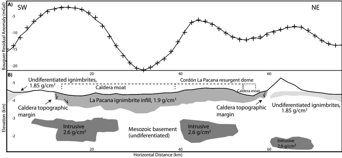
FIG. 4. Forward model of the SW-NE cross section. **A.** Bouguer residual anomaly (crosses) and model prediction (continuous line); **B.** Topography (negative above sea level) and model geometry. Numbers are the densities used in the forward modeling. Arrows in the intracaldera infill are interpreted as normal faults in the caldera hanging wall. Dashed lines delimit the caldera moat and resurgent dome. See text for details.
