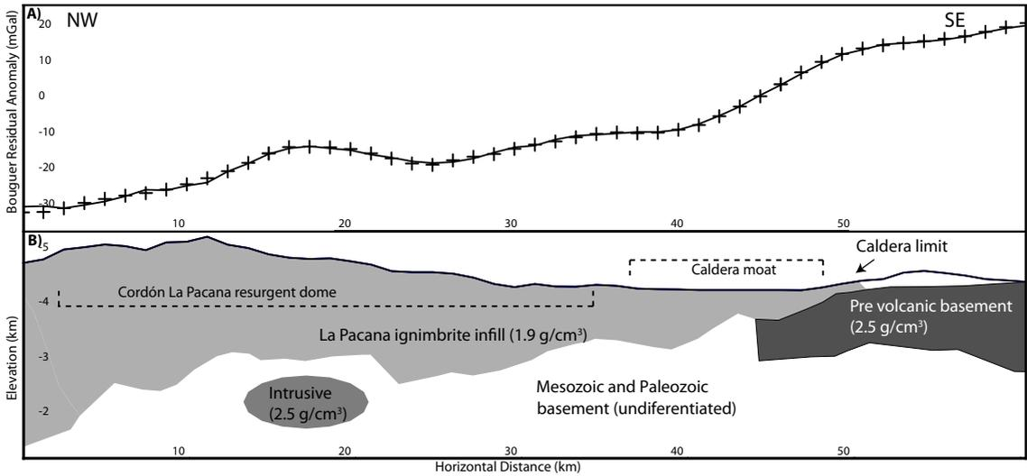
FIG. 5. Forward model of the NW-SE cross section. Legend as in figure 4.
