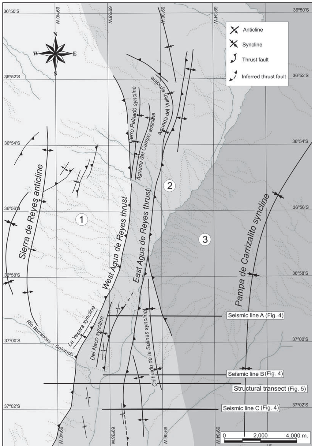
FIG. 3. Main structures described in this work. Note three different zones (1, 2, 3). Zone 1 has a broad discontinuous structure; zone 2 has longer and narrower structures with a shallower décollement; zone 3 is represented by the broad Pampa de Carrizalito syncline. Locations of seismic lines of figure 4 are indicated, as well as structural section depicted in figure 5.
